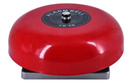
Operating Voltage - DC 12V, 24V, AC 110V, 220V Volume decibel - ≥110dB Protection level - IP45 Dimensions diameter Ф250mm × Height 70 mm Appearance Material - alloy
